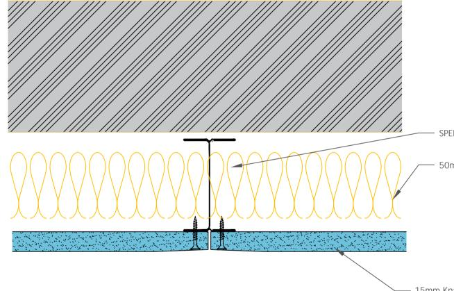
SPEEDLINE 70mm 'I' Studs at 600mm Ctrs
